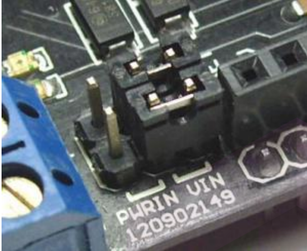
Figure 5 The motors are powered by Arduino power supply
